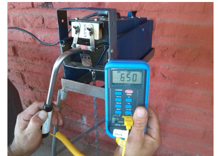
Pyrometer indicating proper blade temperature of 650°C.
