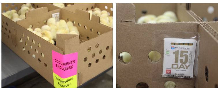
Chick box temperature recorders monitor temperature during transportation from hatchery to breeder farm.
