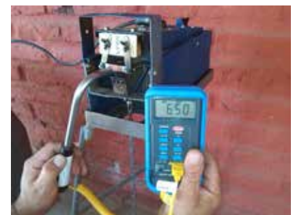
Pyrometer indicating proper blade temperature of 650°C.
