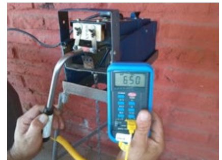
Pyrometer indicating proper blade temperature of 650°C.
